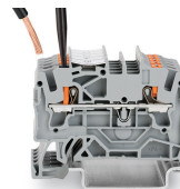
Insert fine-stranded conductors via operating tool.
