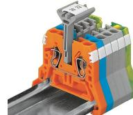
In addition to the plastic marker strips, group marker carriers are now available for the WMB and WSB marking systems. They can be mounted in parallel to a push-in type jumper bar via the open jumper contact slot. It is also very useful if the marker slots on the side of the terminal block are hidden. The carriers are available in the following widths: 5 mm (0.197 inch), 10 mm (0.394 inch) and 15 mm (0.591 inch).
