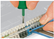
Inserting/removing a conductor – 256 Series.
