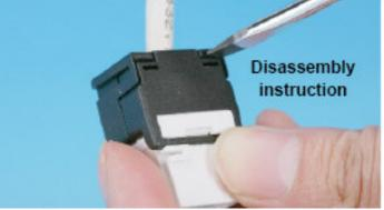
In order to open the connector clip, horizontally insert a screwdriver into the top horizontal slot and rotated it for loosing one side. Then insert this screwdriver by the same way to the slot in the other side. Rotated it until the cap opens.
