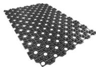
Thermoformed, perforated mat for low-profile underfloor heating with the usage of special underlays. The mat allows to assembly a wet-built floor covering up to 3 cm high. The underfloor heating system is dedicated to renovated buildings and other buildings where the technical conditions make it impossible to perform underfloor heating in a traditional form.
