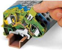
Commoning ground conductor terminal blocks with through terminal blocks is possible in one direction only (via rear side of terminal block) using adjacent jumpers. WAGO recommends using yellow-green adjacent jumpers in addition to the required marking of these blocks.
