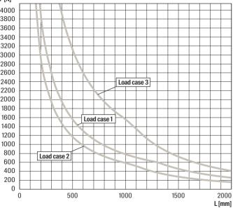
For the load curves, the permissible steel strain  $\delta_{adm.} = 188$  N/mm (increased steel strain due to bending)and the maximum deflection under load L/200 are not exceeded. Fixings and screw fastenings must be calculated accordingly. The higher yield strength is a result of the calculation according to DIN EN 1993-1-3:2010-12, para. 3.2.2.
