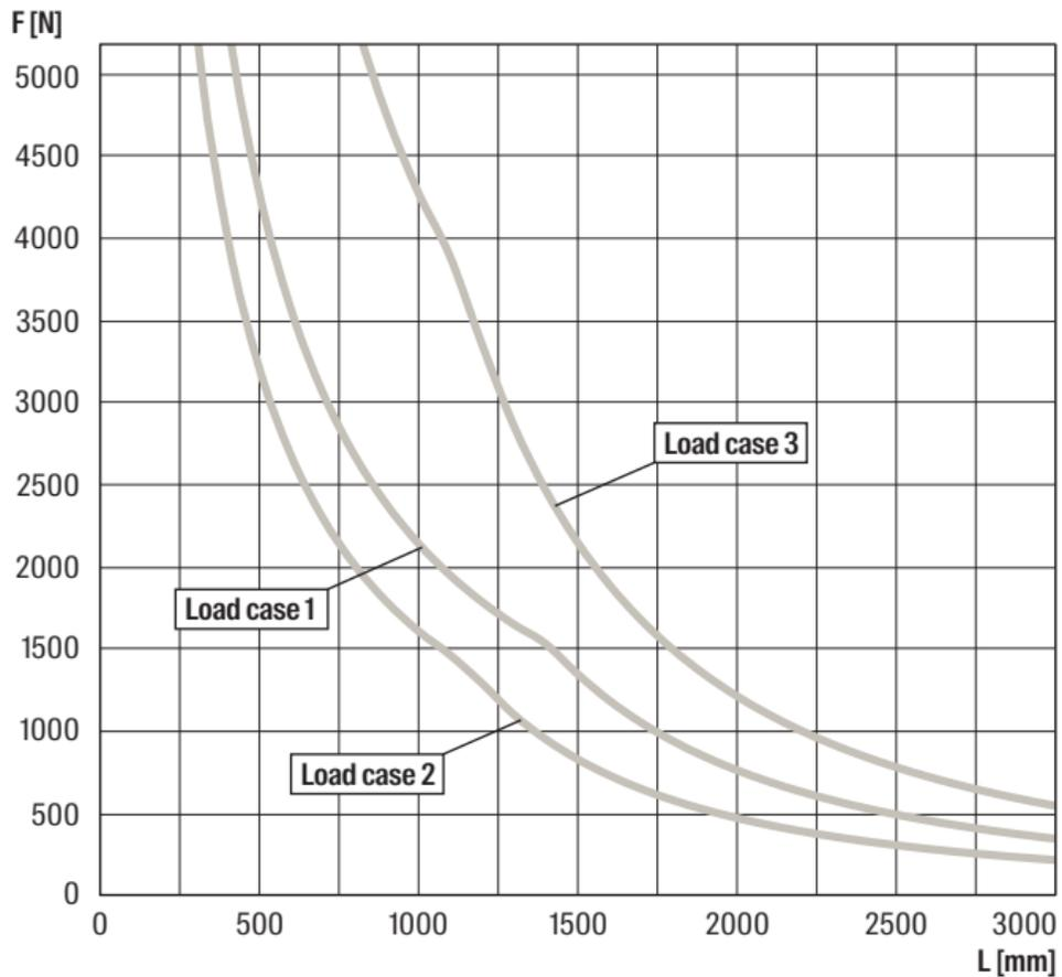
For the load curves, the permissible steel strain  $\delta_{adm.} = 188$  N/mm and the maximum deflection under load  $L/200$  are not exceeded. Fixings and screw fastenings must be calculated accordingly. The increased yield strength is calculated according DIN EN 1993-1-3:2010-12, sec. 3.2.2.
