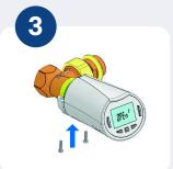
Fix the two screws to the brackets
