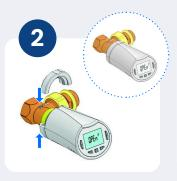
Fix the brackets to the adapter nut and the head
