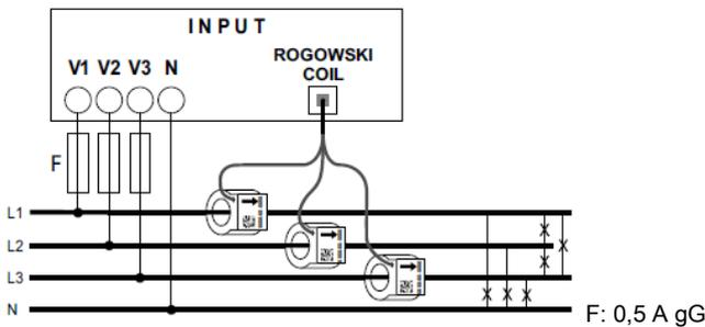
. Rogowski coil(s) cable length (see § Overall Dimensions) allow you to put EMS CX<sup>3</sup> Measure modules everywhere in the installation. This is not mandatory to have them near to the associated protection device of the measured line.
