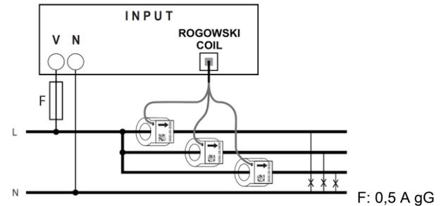
**Note: the 3 single-phase circuits measured must come from the same phase.**
