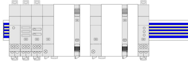
**Implementing:** with this configuration, the plastic protection cover of the backside communication ports on the EMS CX<sup>3</sup> module must be removed.
