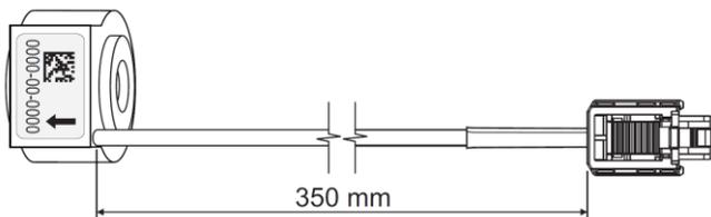
This length can be stretched via the Extension cable + connector up to 3,35 meters (0,35 m of Rogowski cable and up to 3 m of extension)
