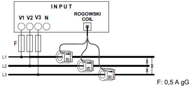
4 wires three-phase network, 3 sensors (3N-3E):
