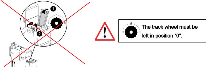
. It is not necessary to address the EMS CX<sup>3</sup> modules. **The track wheel must be left in default position "0".**
