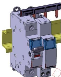
2. Pull the device forward in order to release it from the rail
