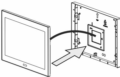
Fig. 15: Attaching the device (example illustration)
