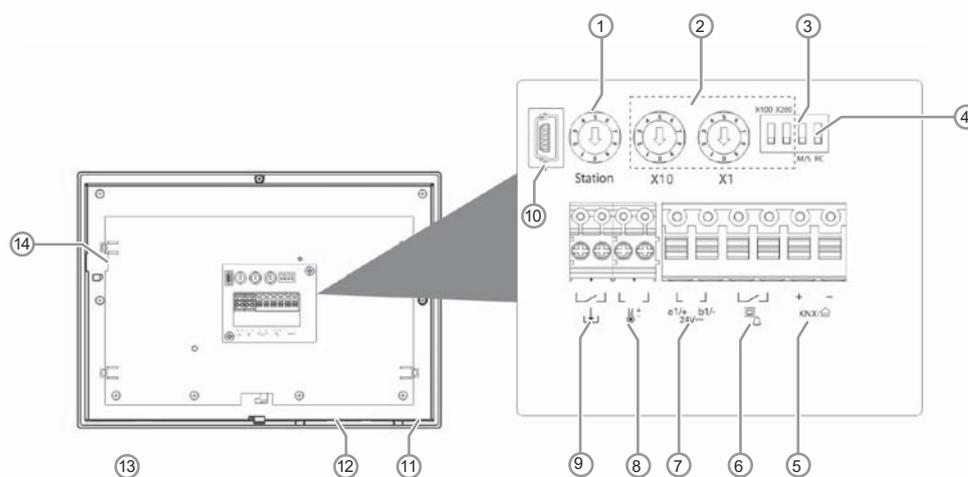
Fig. 3: Device overview Busch-SmartTouch® rear side
