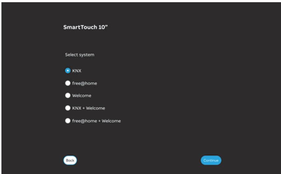
Fig. 18: Selection of system during initial commissioning
