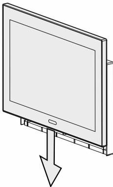
Fig. 16: Latching the device (example illustration)
