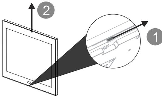
Fig. 17: Loosening the clamp of the device
