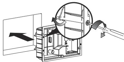
Fig. 9: Mounting in hollow wall
