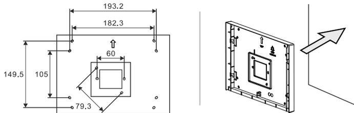
Fig. 10: Installation of surface-mounted mounting frame
