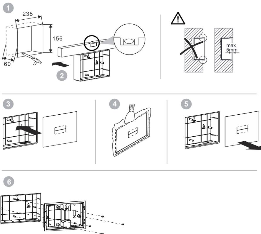
*Fig. 8: Mounting in solid wall*
