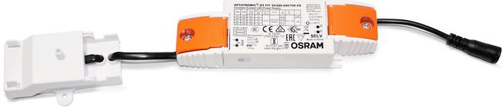
Osram OT FIT 30/220...240/700 CS driver set up at 700mA current with DC cable and LiLo box to connect to OptiClip light engine kit
