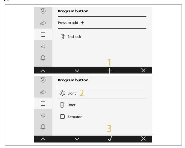
If the function is set to "Light", "Door" or "Actuator", you need to select the address.
