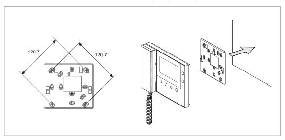
3. Surface mounted with the electrical accessory box (unit: mm)
