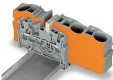
Step-down jumpers common terminal blocks of different sizes, without losing a conductor clamping point. This can be beneficial on long conductor runs where voltage drop can be a problem. A large conductor can be easily connected to smaller conductors at the distribution point.
