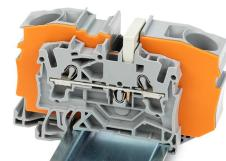
**Step-down jumper (2016-499)** commons 16/10 mm<sup>2</sup> (16/8 AWG) terminal blocks (2016/2010 Series) with 10/6/4/2.5 mm<sup>2</sup> (8/10/12/14 AWG) terminal blocks (2010/2006/2004/2002 Series).
