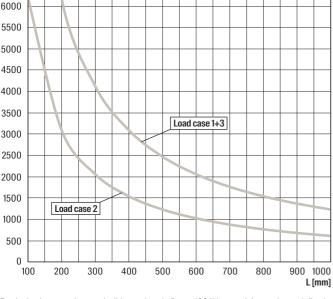
For the load curves, the permissible steel strain  $\delta_{adm.}$  = 160 N/mm and the maximum deflection under load L/150 are not exceeded. Load values of the cantilever arms under consideration of the load capacity of the base plate. Fixings and screw fastenings must be calculated accordingly. The load curves are valid for all material thicknesses of the FCA brackets.
