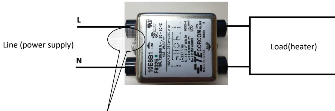
Please make sure the PE contact of the filter is on the side of the power supply (line)!
