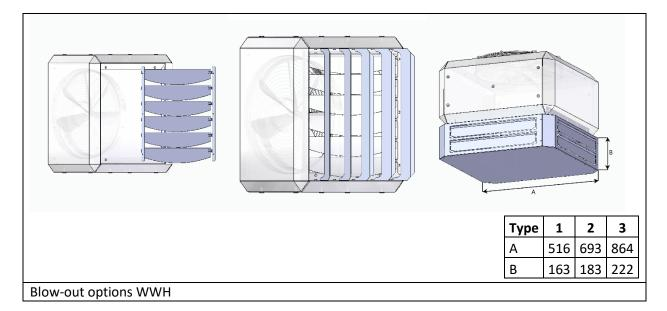
The discharge grille, 4-sided discharge plenum and the vertical blades can be easily removed and directed to the desired discharge direction. When using a plenum, the throw decreases by a factor of 4! Make sure that the exchanger is not damaged at all times.
