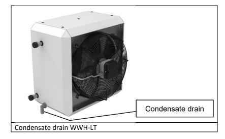
**Wall setup:** The pipe connections for water should always be **horizontal**, with a view to venting of the internal pipes. The heater can be turned over slightly, but the heater may absolutely not hang askew. Place the heater in such manner that, the supply connection (hot water) is at the lowest point. It's important to place the venting in the duct near the heater.
