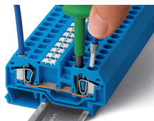
CAGE CLAMP® connection Inserting a conductor. With ferruled conductors, it is necessary to use a terminal block one size larger than the conductor's nominal cross-section.
