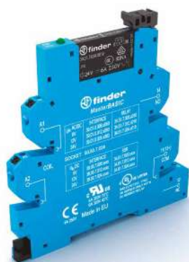
Type 39.01.0.024.0060 1 wisselcontact 6 A 250 V AC1
