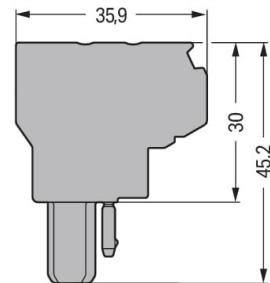
$L = \text{pole no.} \times \text{module width}$
