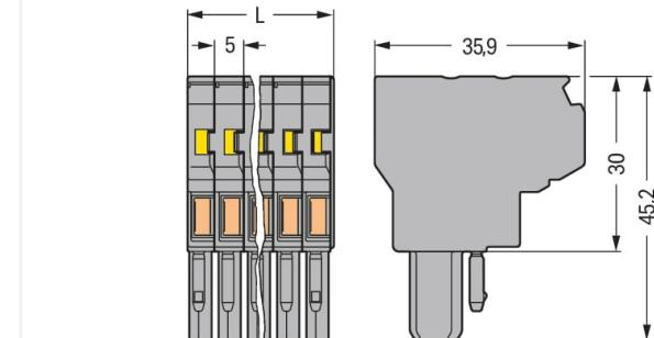
$L = \text{pole no.} \times \text{module width}$
