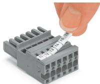
Labeling a female plug with CAGE CLAMP® connection via Mini-WSB Quick Markers.
