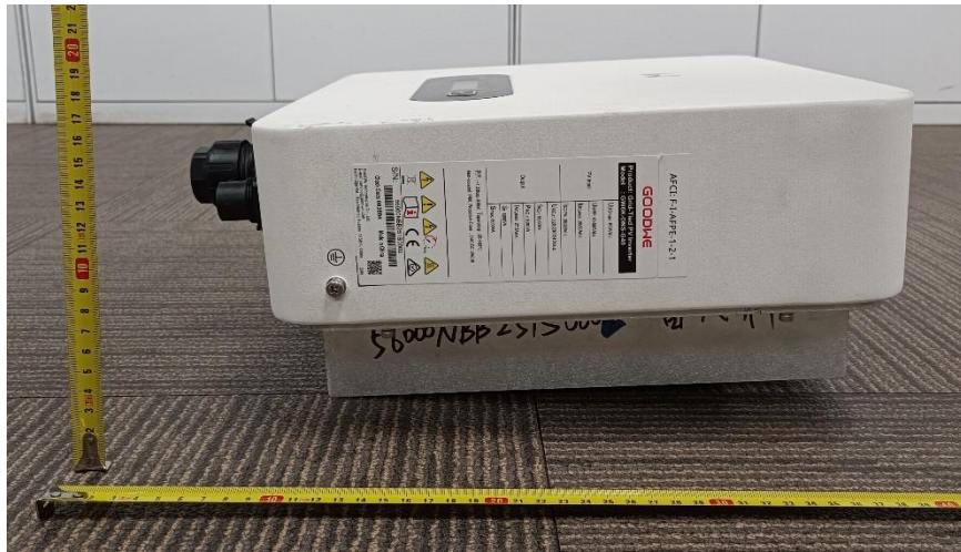
Figure 9. External earthed terminal view
