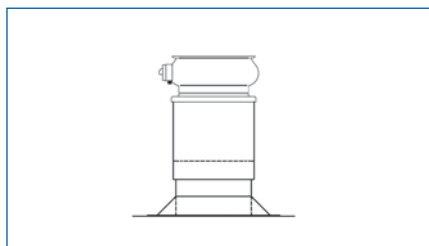
Dakventilator, geluiddemper, dakopstand
