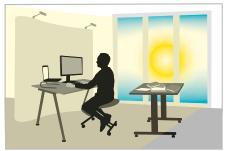
Movement/presence detected but with sufficient brightness the 18.51 keeps the lamps Off.
