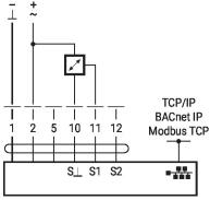
TCP/IP (Cloud) / BACnet IP / Modbus TCP with analogue setpoint (hybrid operation)
