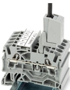
Testing tap (Item No. 2009-182) for tool-free connection of test cables up to 2.5 mm² (12 AWG) – compatible with 2000 to 2016 Series
