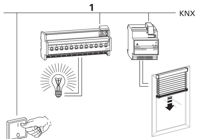
Push-button action to OFF=> telegram value "0" => light OFF and retrieve preset position 1 = open roller shutter:
