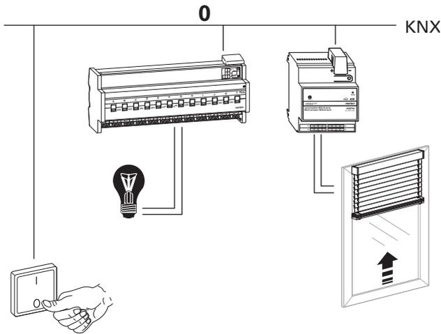
In this case, due to the fact that the roller shutter requires a certain running time to open, the light needs to be switched off with a switch-off delay so that it doesn't suddenly become dark prematurely.
