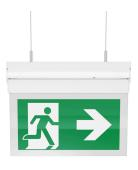
LiFeSafe PRO MULTIFIX EX SUS EM3 NM/MT DA is a DALI addressable LED ceiling suspended exit sign complete with six ISO7010 legends: Left, Right, 2 x Up and 2 x Down. Maintained or Non-Maintained, 3Hr emergency duration. Maximum viewing distance 28m. 0 to +35°C operating temperature range. IK02, IP65, Class II electrical construction, 6-year warranty.
