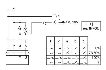
Override control with AC 24 V with Control remotely 0...100% with
