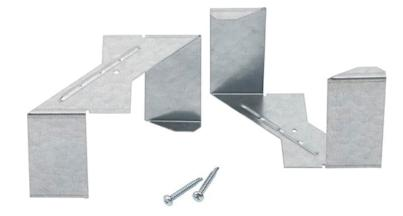
Mounting bracket for Optix Linear Recessed range. Suitable for ceiling thickness 1-20mm. Contains 5 pairs of brackets suitable for fixing 5 luminaires. Necessary screws are included in the pack.
