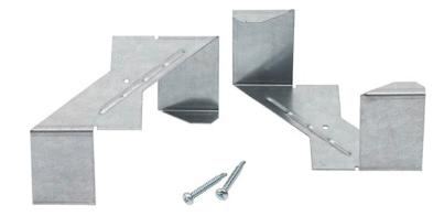
Mounting bracket for Optix Linear Recessed range. Suitable for ceiling thickness 21-40mm. Contains 5 pairs of brackets suitable for fixing 5 luminaires. Necessary screws are included in the pack.
