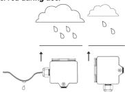
Regardless of the compass direction, the outdoor sensor should not be mounted in the following locations:
