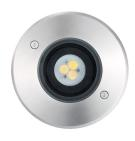
• Round shaped in-ground luminaire with +/-30° adjustable light module, drive-over for pressure loads to 2000kg (20kN), comes with 2m 3x1mm2 flying lead and recessing tube, aluminium housing with Stainless steel (SS316) decorative ring and clear glass diffuser, IP67, IK10, Class I, non-dimmable, 390lm, 5.7W, 68lm/ W, CRI80, 30° beam angle, 50000 hrs L70 B50 lumen maintenance, 120mm diameter, 136mm recessing tube height, 0.81kg weight.
