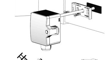
The sensor can be mounted on the ventilation duct by means of the mounting clip. For risk of condensate permeation in the sensor tube respectively in the immersion pocket the bushing must be installed in a position that occurred condensate can run off.
