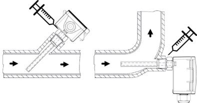
Mounting with immersion pocket or compression fitting for usage in liquid media. Use contact fluid for better heat transfer between sensor and measuring medium.
