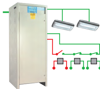
Failure of normal lighting final circuit
