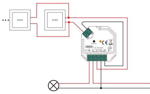
This phase dimmer adopts trailing edge dimming (reverse phase control), please make sure the connected loads support reverse phase control. Please refer to the user manual of the load or consult the supplier of the load.
