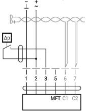
Switching contact requirements: The switching contact must be able to switch a current of 16 mA at 24 V accurately. Start point of the operating range must be parametrised on the MOD actuator as ≥0.5 V.
