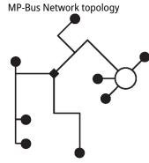
There are no restrictions for the network topology (star, ring, tree or mixed forms are permitted). Supply and communication in one and the same 3-wire cable • no shielding or twisting
