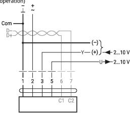
Connection with switching contact, e.g.  $\Delta p$  monitor
