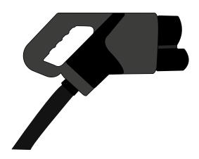
Type CCS, marked with the letter "K", is located on the left side of the charger. The CCS gun is automatically released/locked by its holster or the vehicle.
