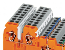
Commoning signal level voltage via insulated push-in type jumper bars (870 Series) – 2- to 9-way, depending on application. Sensor LED terminal blocks cannot be commoned!
