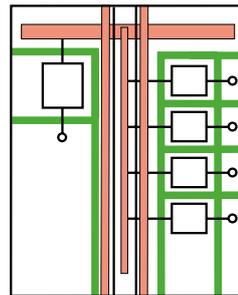
Terminals for external conductors not in the same compartment as the associated functional unit, but in individual, separate, enclosed protected spaces or compartments.
