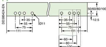
Drill hole dimensions for 10 mm thick horizontal busbars.
