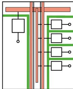
Terminals for external conductors in the same compartment as the associated functional unit.
