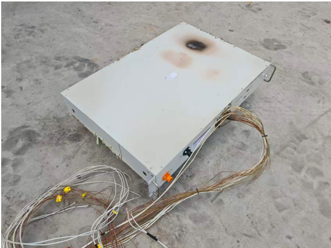
Figure 33. Photo 1 of initiating module after test
