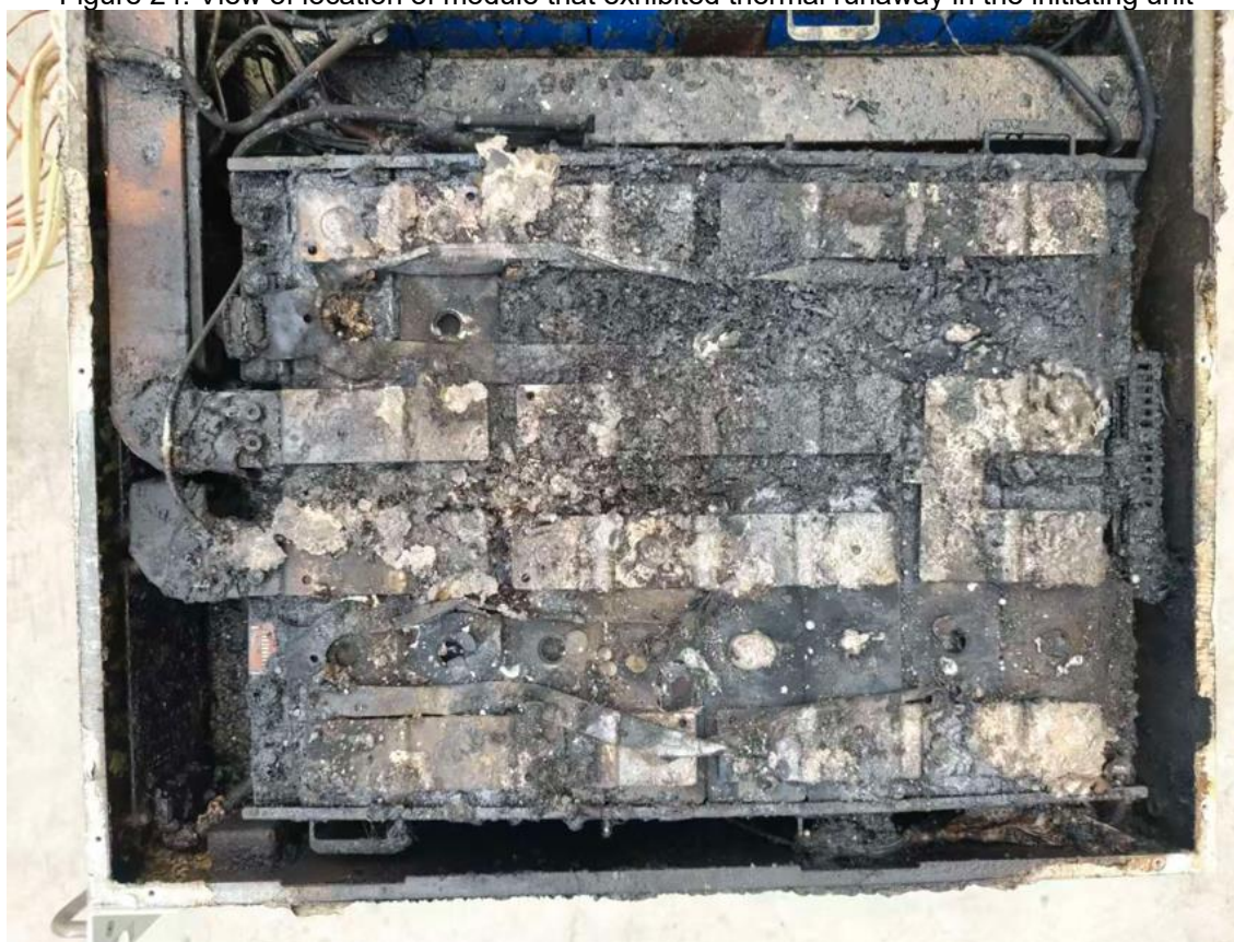
Figure 25. View of location of cells that exhibited thermal runaway in the initiating module
