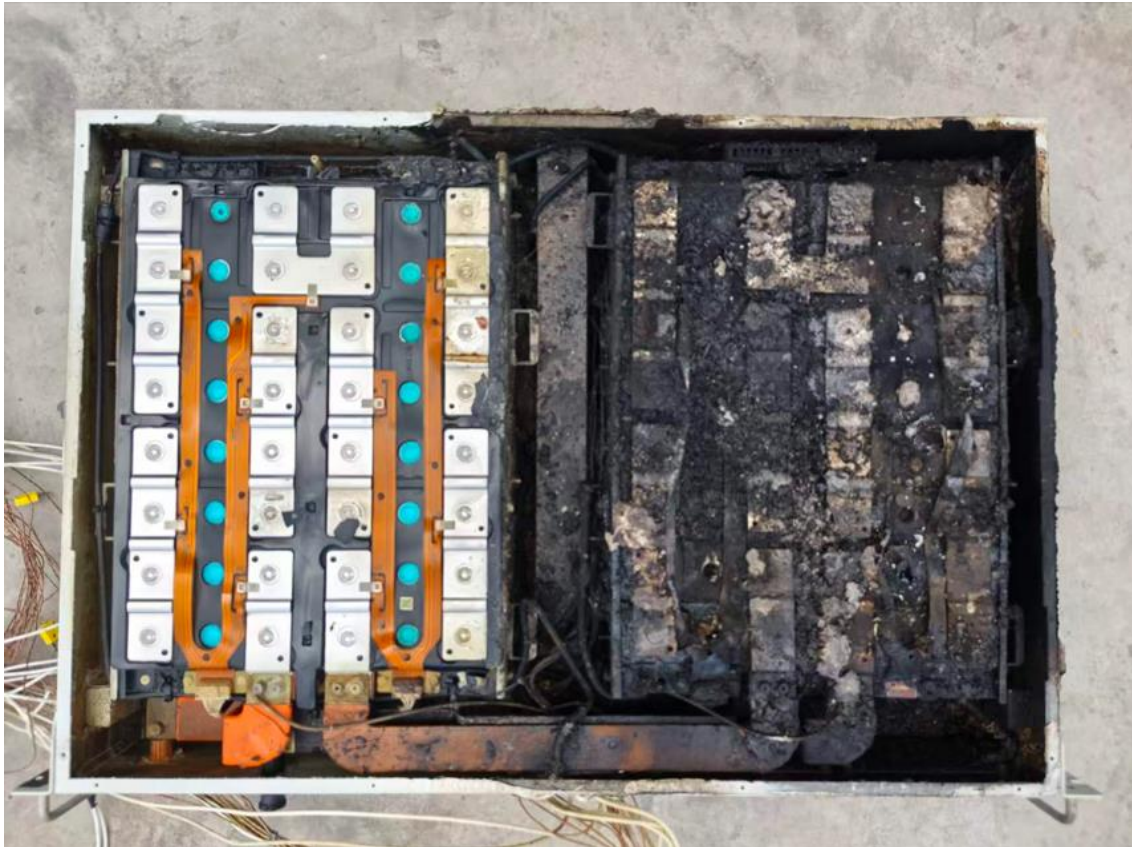
Figure 35. Photo 3 of initiating module after test
