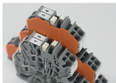
Created for double- and triple-deck TOP-JOB® S Terminal Blocks, the vertical jumpers can common two or three levels. Clearly marked numerals ("2" and "3") distinguish the double-deck (Item No. 2002-0492) and triple-deck vertical jumpers (Item No. 2002-0493), even when inserted.
