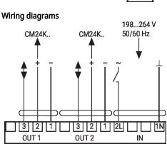
The module can also be operated with only one damper actuator.
