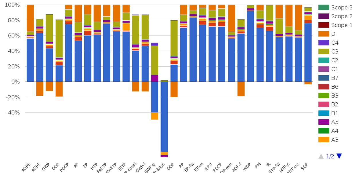
The most significant contribution is from the raw materials in A1. This is offset by the contribution (benefit) in module D. The metal (copper) is very well recyclable and because of its value it is always recovered. The plastics in the product are recovered from production waste, but not End-of-life. Because there is no return program for the product end-of-life the default EOL scenario's are used and these still consider mostly incineration as EOL process.
