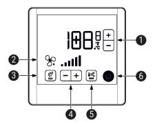
Temperature setpoint: Set the desired temperature
