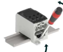
Removing from DIN-rail Release the slider part with a screwdriver. Lift the connector.
