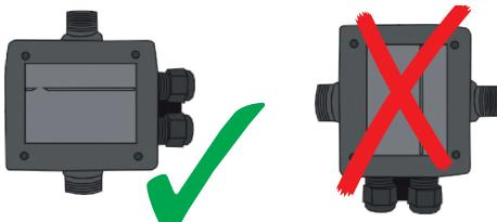
For use with a submersible pump, do not install in the pump tank:
