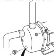
If the system is not to be used for an extended period, drain the pump, clean it and store it (see 2.3).
