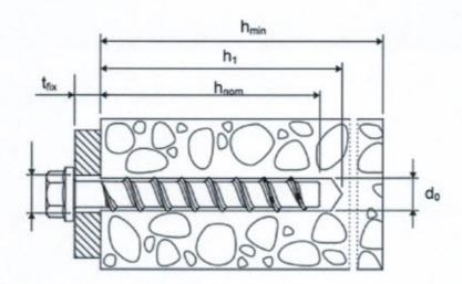
d<sub>0</sub> = nominal drill bit diameter h<sub>nom</sub> = nominal anchorage depth h<sub>1</sub> = depth of the drill hole
